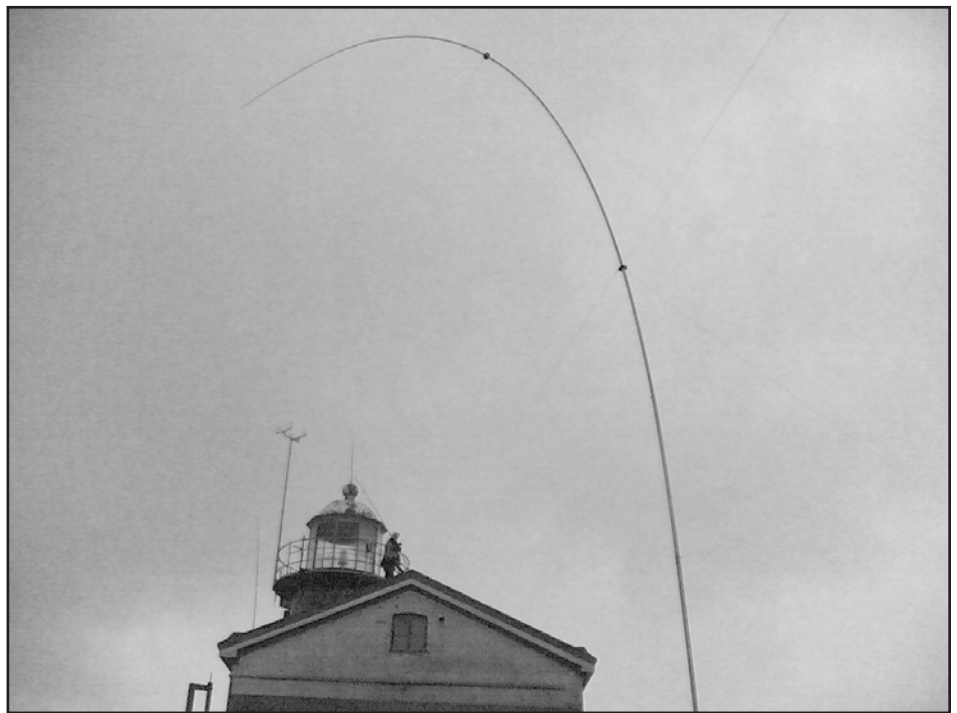
No wonder aluminum of U.S. origin can take a lot of hits. Our thanks to Rich, K7ZV, who provided two of these verticals. We found rolling waves made those guy wires loose — the vertical was “fishing” but did not break.
