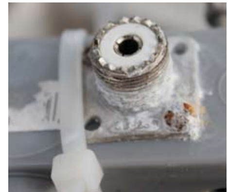
Corroded connectors after 10 days in the sea. A very small price for extra db.
