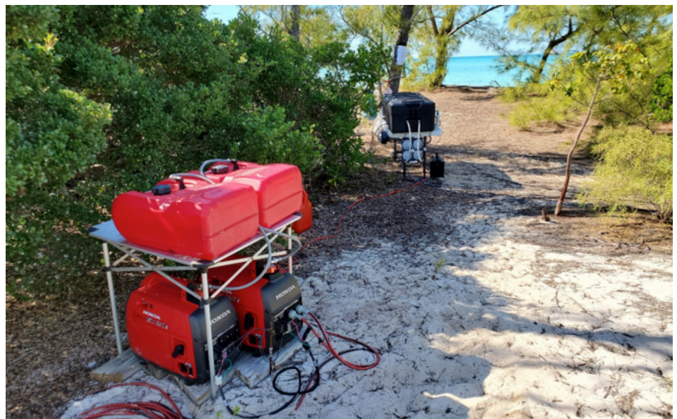
The RIB contains special features that allow the entire 1kW station to run on this efficient and low fuel consumption generator. Note the extended fuel tanks that allow up to 36 hours of operation on a single fill. Fewer visits to the island!
