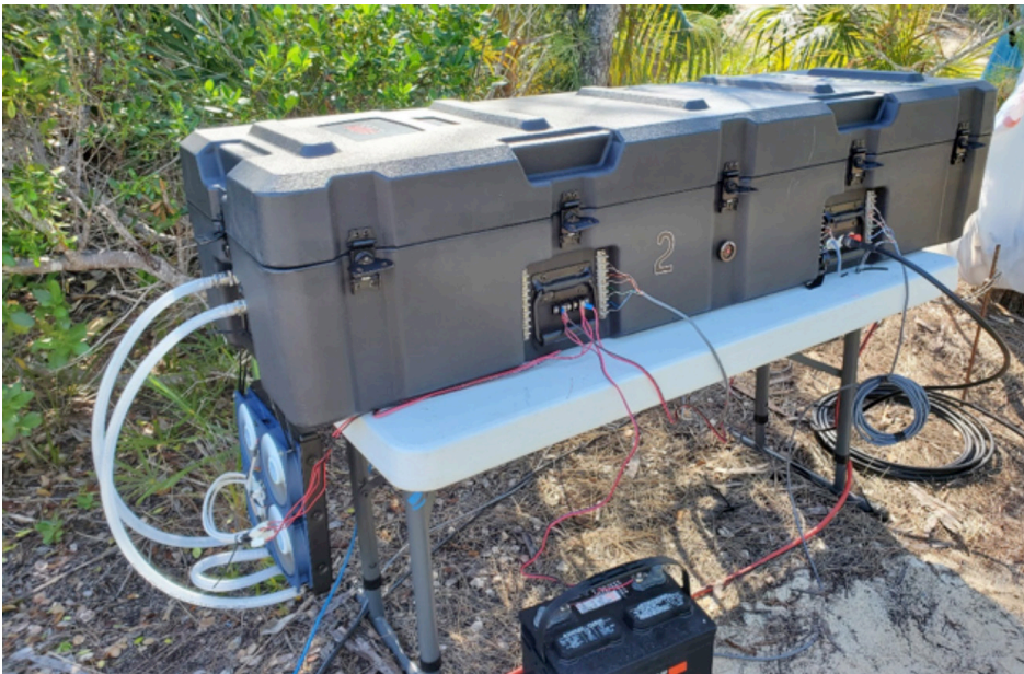
RIB on Water Cay, Bahamas. Note the external cooling radiators.
