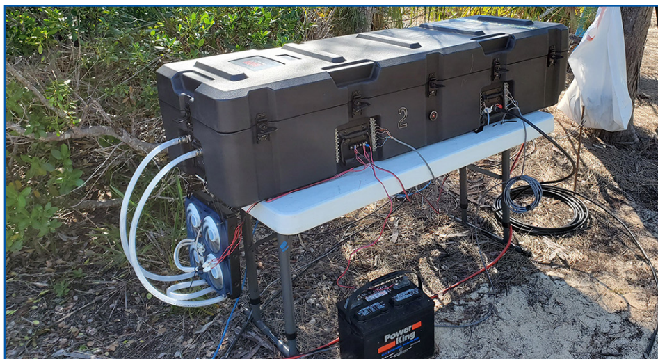
The RIB is a complete station — including transceiver, amplifier, power supplies, cooling systems, and electronic controls — all in a weathertight box.
